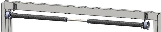
There are only two bolts for each hanger, compared to four for the traditional systems. Also, there is only one hand to the bracket. Since the bracket feet are covered by the spring system, there is no need for a right and a left, reducing part numbers.
